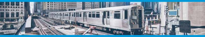
Holland's TrackSTAR® testing vehicles can simultaneously collect track geometry, track strength, and rail profile measurement data to provide a comprehensive assessment of your track condition.
