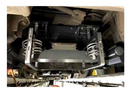
angle. The system utilizes locomotive power, reducing the overall cost and minimizing the number of components to maintain. Proprietary mounting and sensor protectors allow maintenance-free operation for a year. Machine-learning based algorithm eliminates false spikes to accelerate turnover time for geometry defects, reports are reviewed remotely by experienced TrackSTAR operators before the delivery to the customer.
