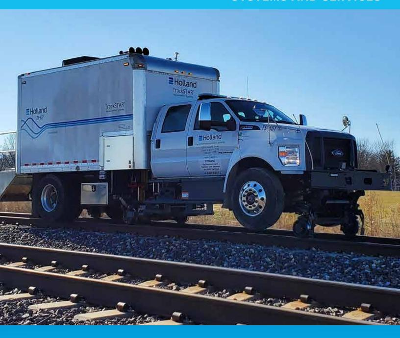
Using Holland's proprietary Argus® track measurement technology, we offer multiple applications to test your track condition.
