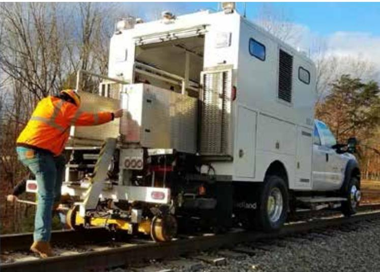
One operator is able to set up and operate the Argus® track geometry system and mini load axle on the NS 02.
