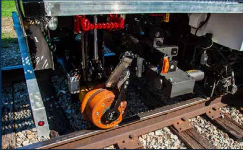
The load axle on the NS 02 generates a consistent 2,500-pound lateral load, a sufficient load for identifying broken spikes.
