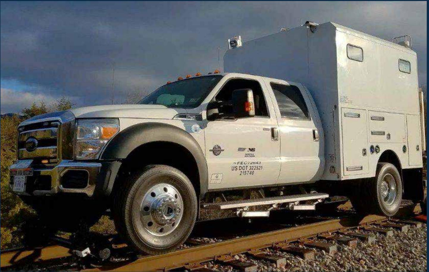
The NS 02 (850-series TrackSTAR® vehicle) will be used systemwide to identify broken spikes.
