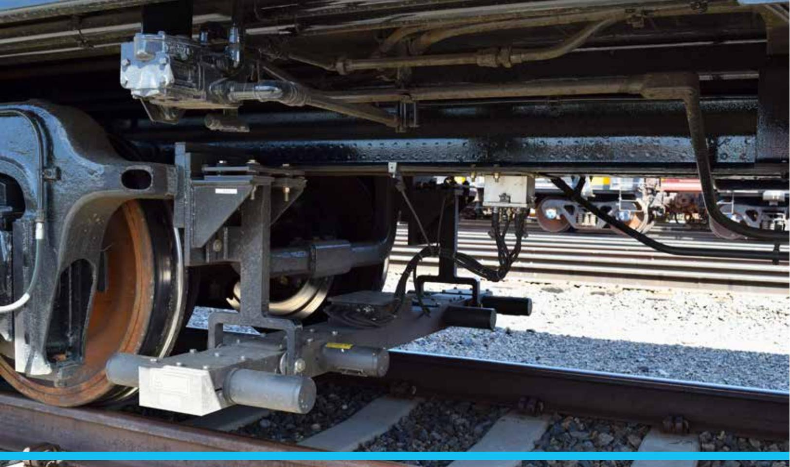
Figure 6 Argus Autonomous Track Geometry and Rail Measurement System
