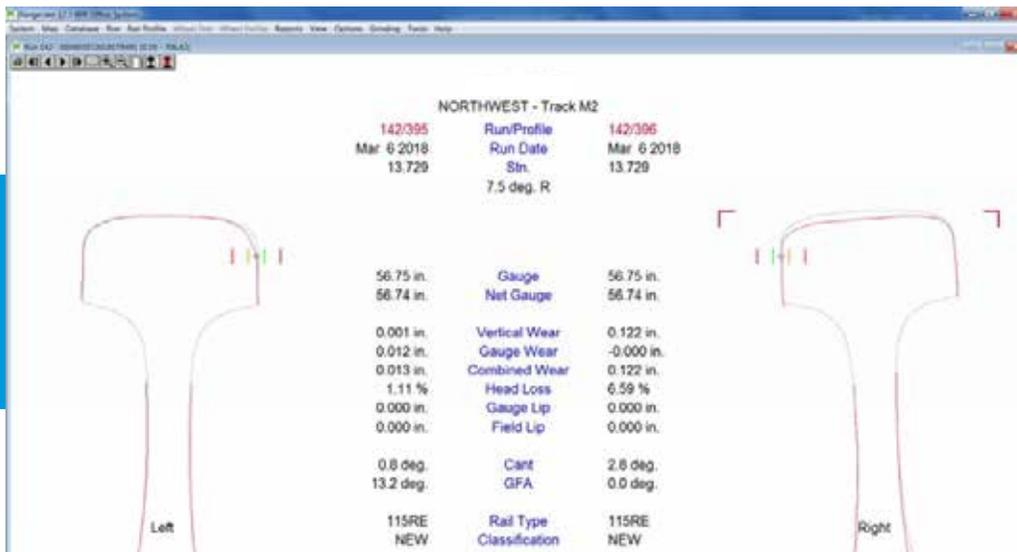
Figure 7 Rangecam Rail Measurement Example with a GFA (13.2° Left Rail, 0° Right Rail)
