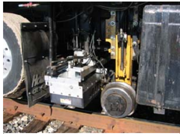
Figure 2. Loaded gauge and geometry measurement at load axle of GRMS test car.
