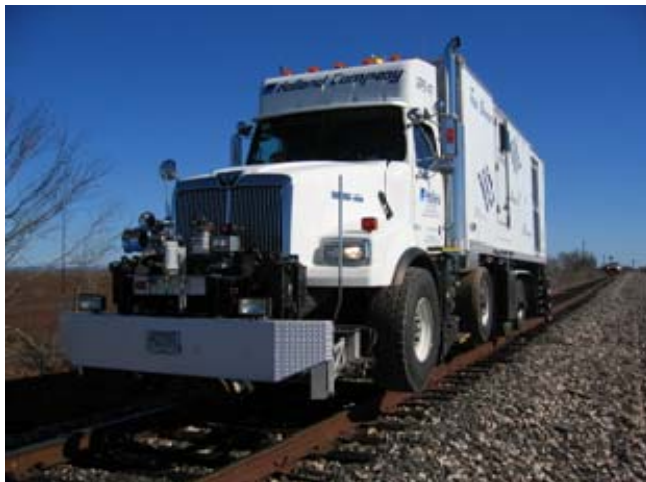
Figure 1. Hi-rail track gauge-strength measurement vehicle (also measures track geometry and rail wear).
