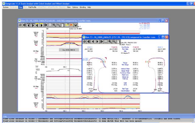
Rail wear profile overlays showing wear over time
