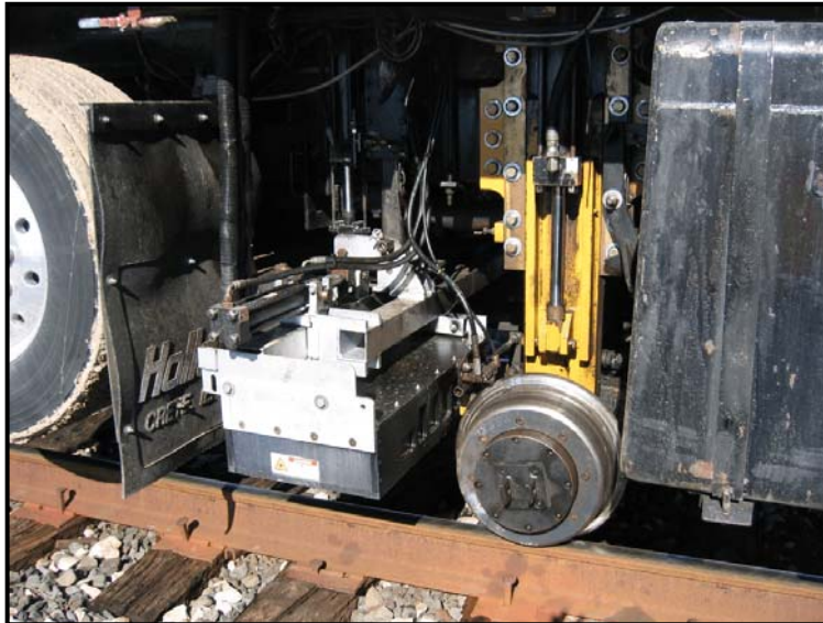
TrackSTAR's split load axle delivers constant, non-destructive vertical and lateral loading
